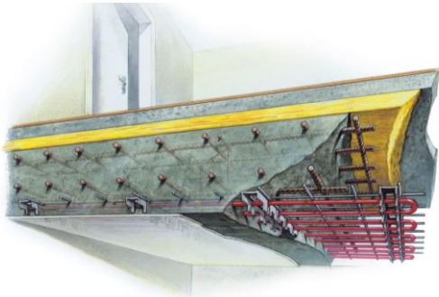
2. Figure: Concrete Core Temperature Control Scheme
